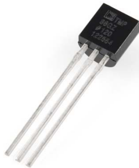
Figure 14: This is a TMP36 analog temperature sensor; it will be used to measure the battery and ambient temperature on the vehicle.
